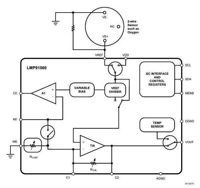
FIGURE 5. 2-Lead Galvanic Cell Ground Referred
