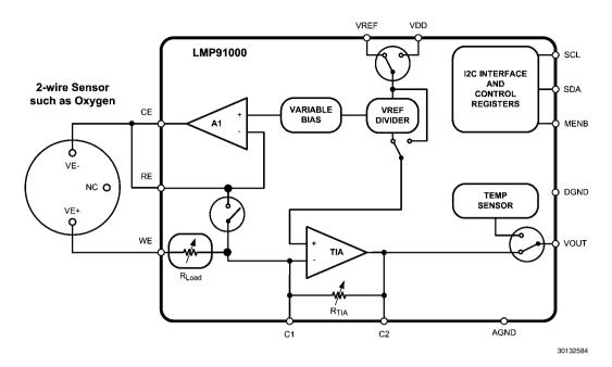
FIGURE 6. 2-Lead Galvanic Cell In Potentiostat Configuration
