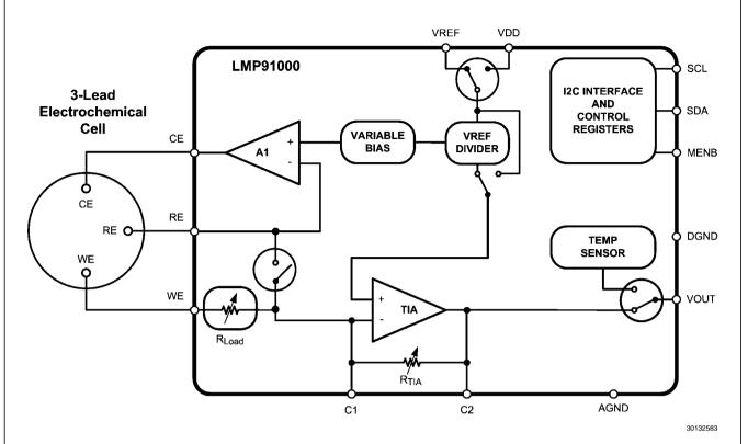
FIGURE 4. 3-Lead Amperometric Cell
