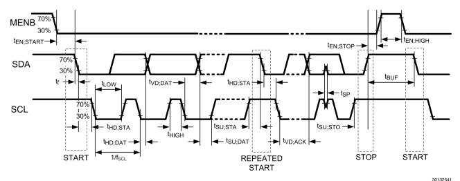
FIGURE 1. I2C Interface Timing Diagram
