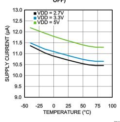
Supply current vs. VDD (Temp Measurement TIA OFF)
