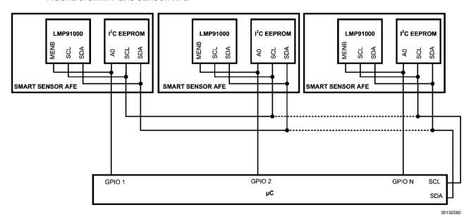
FIGURE 9. SMART GAS SENSOR AFEs on I<sup>2</sup>C bus
